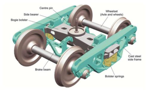
The subjects of truck design and rail-wheel interface are quite complex.<sup>10</sup> For present purposes, I will only say that there are substantial advantages to the classic, symmetric designs, used for conventional railcars. These have a frame and two pairs of wheels, each pair joined by an axle. A principal advantage of this arrangement is self-steering when running in either direction, *i.e.*, an inherent ability of the truck to follow the tracks and not derail.<sup>11</sup>
