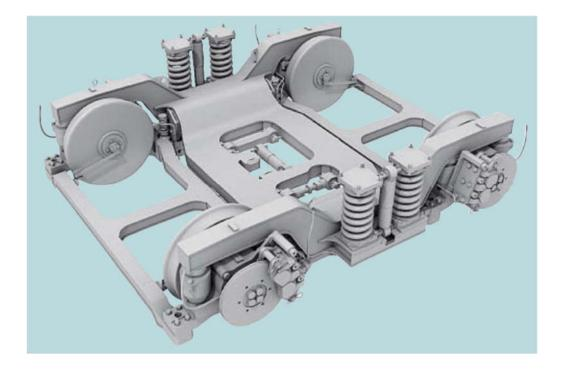
Some truck designs for very low-floor trams have proved unsuccessful. As Megna *et al* stated, "vehicles with steering axles and independently rotating wheels, which could be the only structural way to eliminate wear and noise problems related to sharp curves, are no longer available on the market, probably because of their lower modularity and high manufacturing and maintenance costs."<sup>14</sup>
