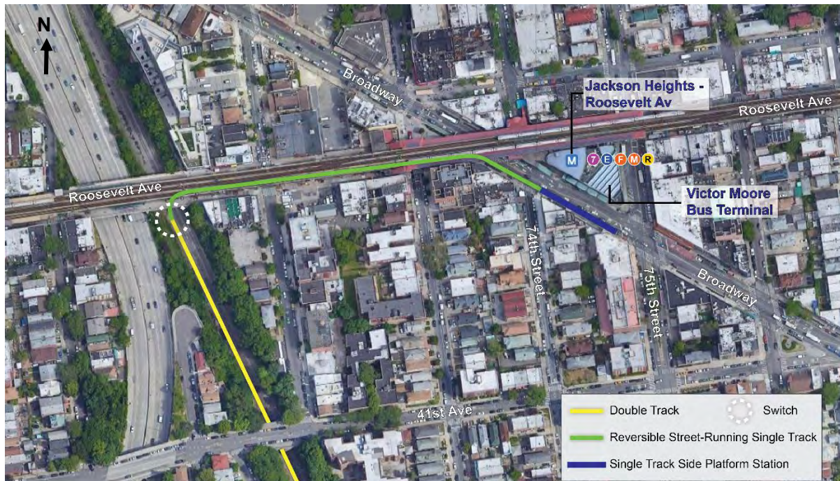
Figure 6: Proposed LRT – Roosevelt Avenue Segment Alignment
